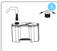
Screw off the the tank cover and add water
